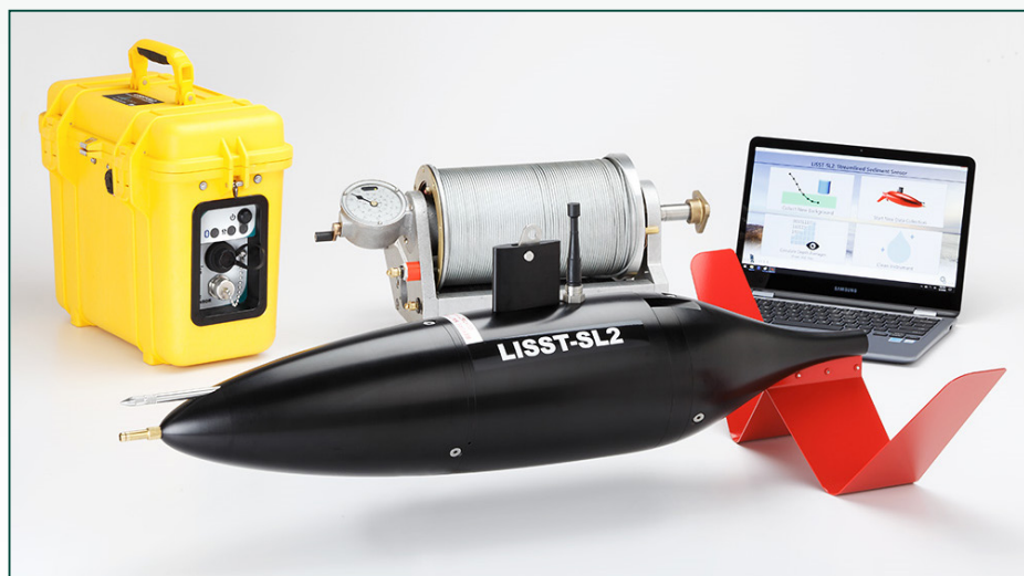
LISST-SL2 with Topside Control Box and USGS B-reel (computer & reel not included)
